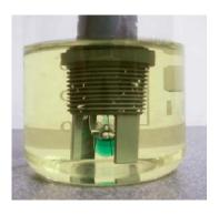
Calibration can be performed using standard pH buffers, usually pH 4, 7 and 10. From the main screen select the pH sensor, press the 'Calibrate' button, and then select 'Calibration'. After choosing whether to calibrate the temperature, as per the instructions above, continue to follow the on screen instructions.
