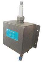
TurbSense turbidity sensor in flow cell
