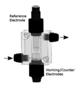
Fig.1 - Non membraned sensor, three electrode potentiostatic system in an acrylic flow cell.
