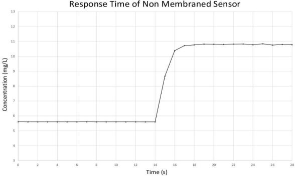
Fig.4 - A graph showing the response time of the non membraned sensor to changes in concentration
