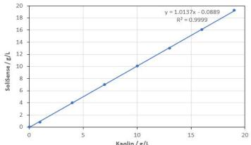
Kaolin/g/L Fig. 5 SoliSense® readings for a range of kaolin samples.
