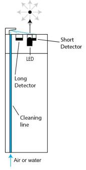
SoliSense<sup>®</sup> uses Pi's novel measurement technique that uses the gradient between the four readings to produce the automated to carry out the cleaning at predefined intervals. sensor output. This configuration allows accurate and reliable measurements of suspended solids concentrations and turbidity to be made.
